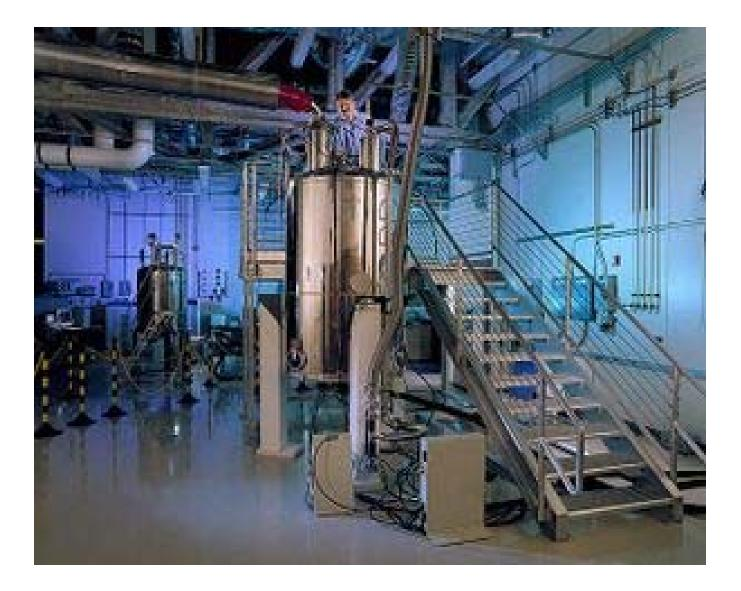
Pacific Northwest National Laboratory's high magnetic field (800 MHz, 18.8 T) NMR spectrometer being loaded with a sample.
