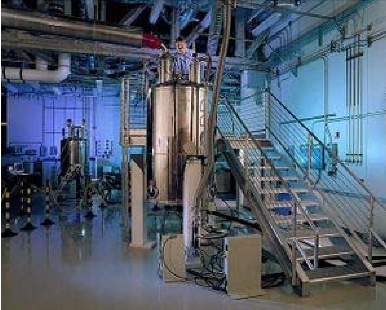
[Pacific Northwest National Laboratory](#)'s high magnetic field (800 MHz, 18.8 T) NMR spectrometer being loaded with a sample.
